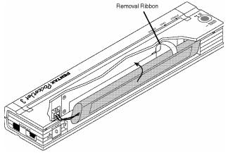
FIGURE 12. Placing the battery inside the battery compartment
